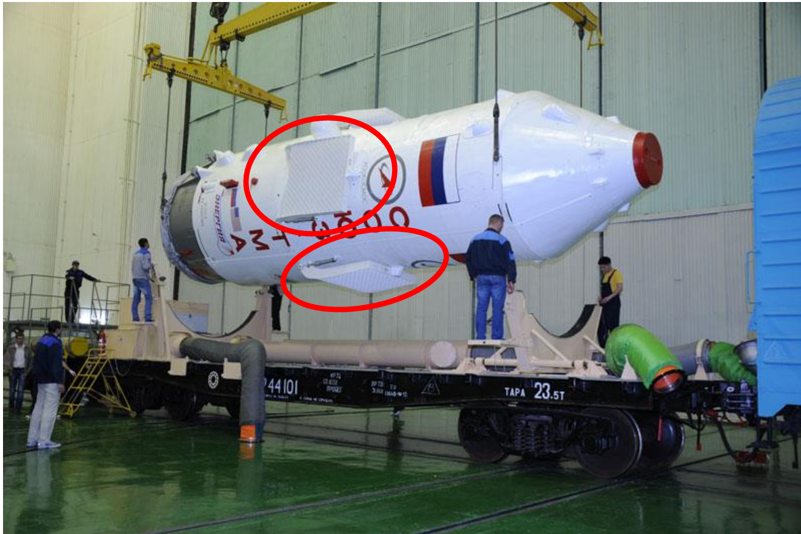
“Encapsulated” Spacecraft transported for integration with LV LES Stabilizer Panels highlighted
