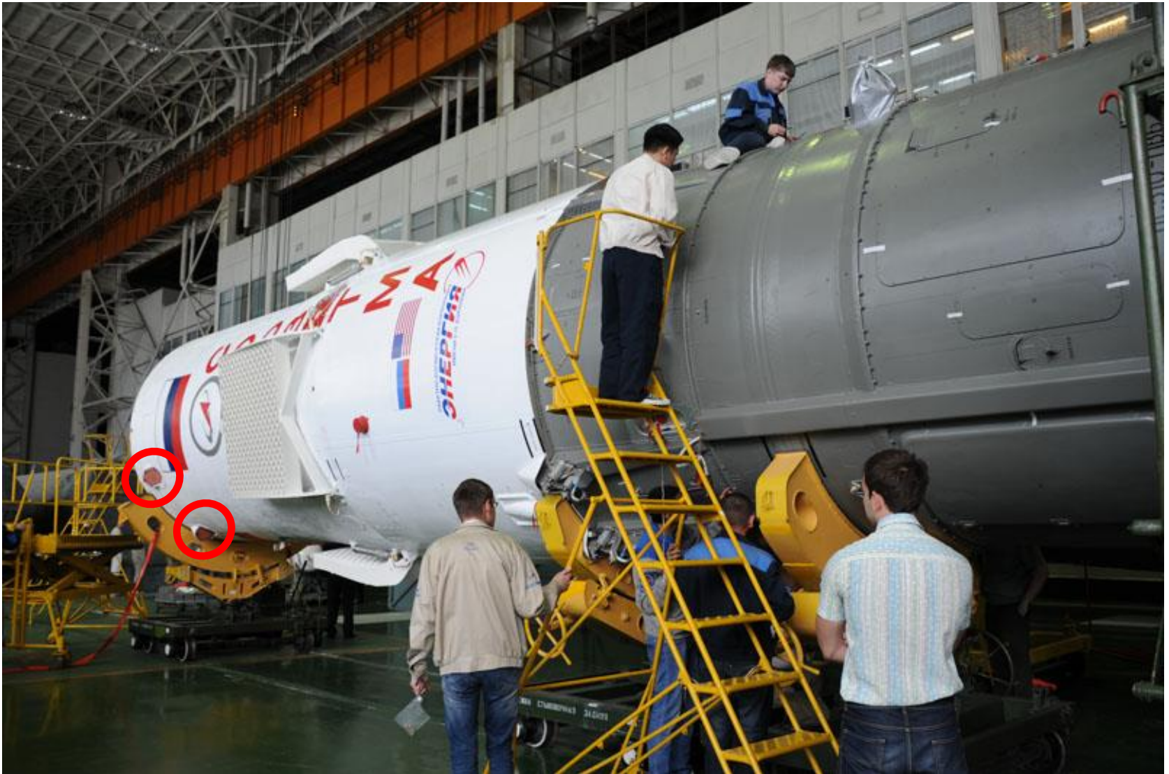
Integration of Spacecraft with 3 rd Stage 2 of 4 Shroud LES rocket nozzles are visible
